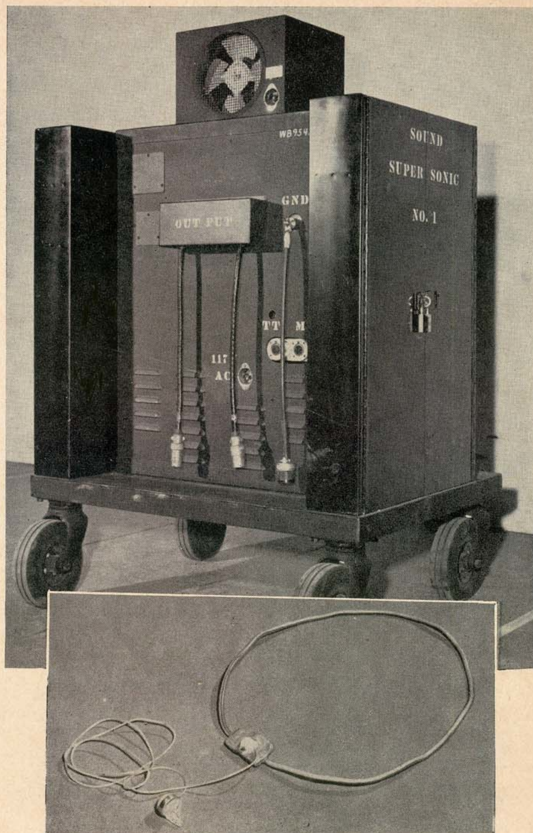
FIG. 2 Warner Bros.' Supersonic Playback Transmitter. Inset shows receiver, loop and earphone.
